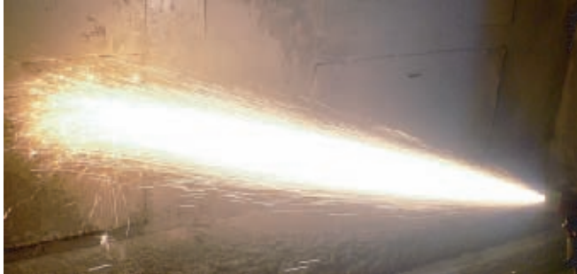
Spraying 1.6mm stainless steel 316L
